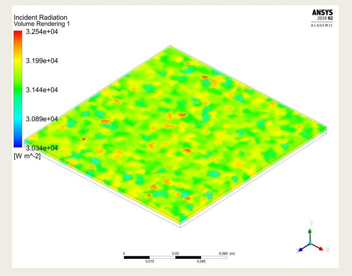
Figure 3: Total Incident Radiation in the Optical Layer when the Radiating Body was at Temperature 295 Kelvin
