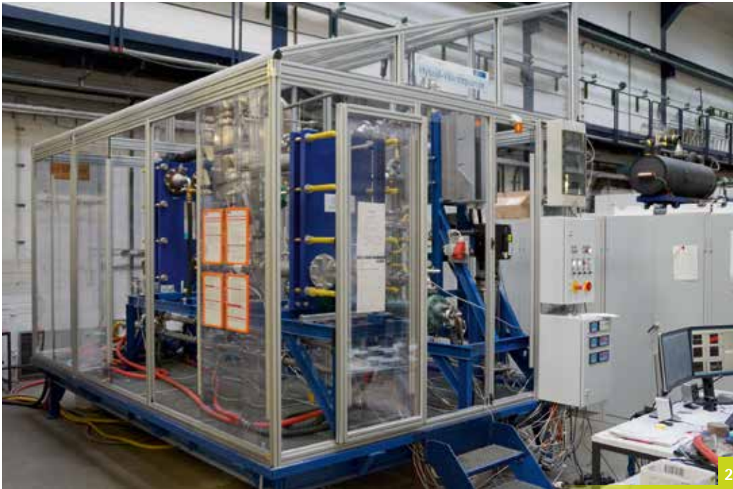
Figure 2 The ammonia/water high-temperature pilot plant at the IfT Photo: IfT
