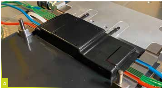
Figure 3 Electronics on the test module before the potting process. Photo: IAL
