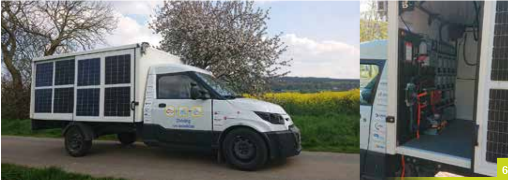
Figure 6 Assembled demonstrator vehicle with lightweight solar module generation. Photo: ISFH
